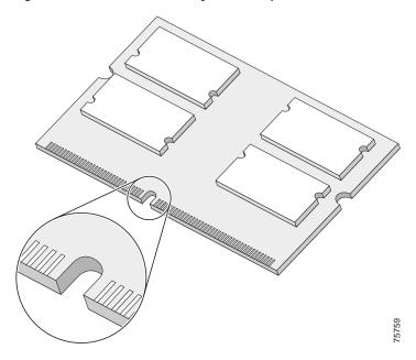
Step 7 The SODIMM must be lined up at a 45-degree angle. (See Figure 56a.)
